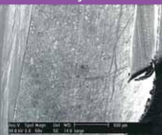
Non-Tulip Reusable Cannula used 5 times. Harvester 3mm, Streaks are believed to be caused by brushing/cleaning process
